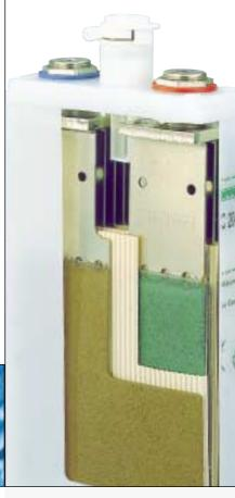
The section of the FNC\* cell clearly shows the corrugated separator between the positive and negative plate.
